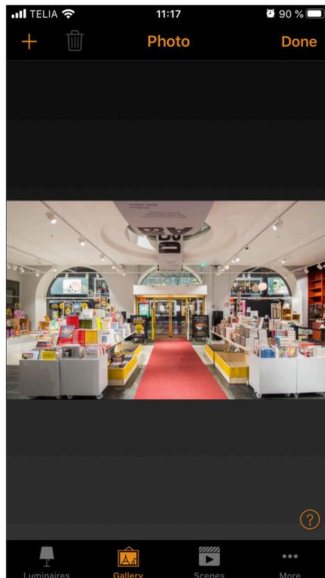
A luminaire control circle is shown in the centre of the image. Drag the control circle on top of the luminaire. You can change the size of the circle by enlarging or reducing the circle using two fingers.
