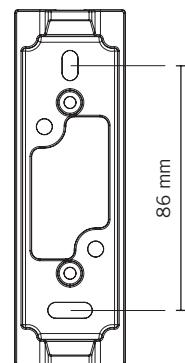
**INSTALLATION AND WIRING - SURFACE MOUNTING**
