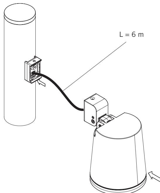
**INSTALLATION AND WIRING - POLE MOUNTING**
