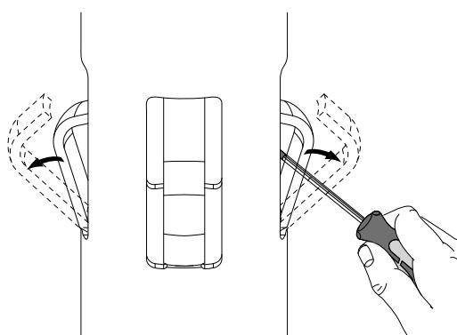
If you need to re-position, bend out the flaps before placing the tube back in the pole foundation
