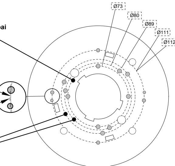
Bracket dismounting: Choose a threaded hole positioned over the foundation
