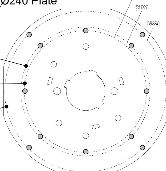
Bracket dismounting: Choose a threaded hole positioned over the foundation
