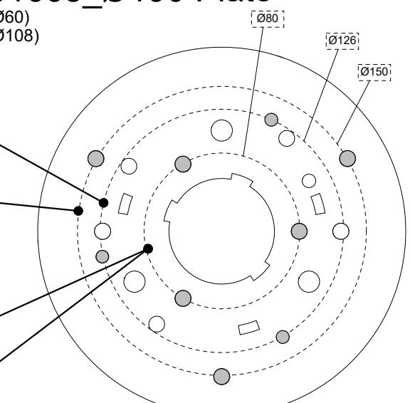
Bracket dismounting: Choose a threaded hole positioned over the foundation
