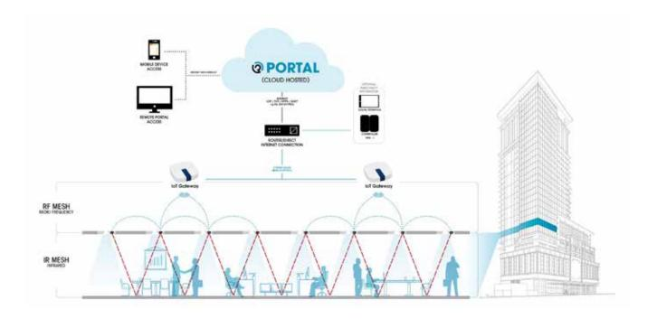
Each IoT-gateway must be in the communications range of at least one sensor node, i.e. within 5 metres in direct view. Each sensor node has the ability to connect to any gateway within the communications range, if there are multiple IoT-gateways close by. An IoT-gateway can in turn be connected to any DHCP network (Building specific) to forward and receive information from the e-Sense Organic Portal.
