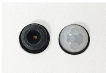
*Light sensor/Switch PIR-sensor*
