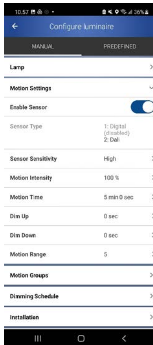
Motion settings - enable sensor.
